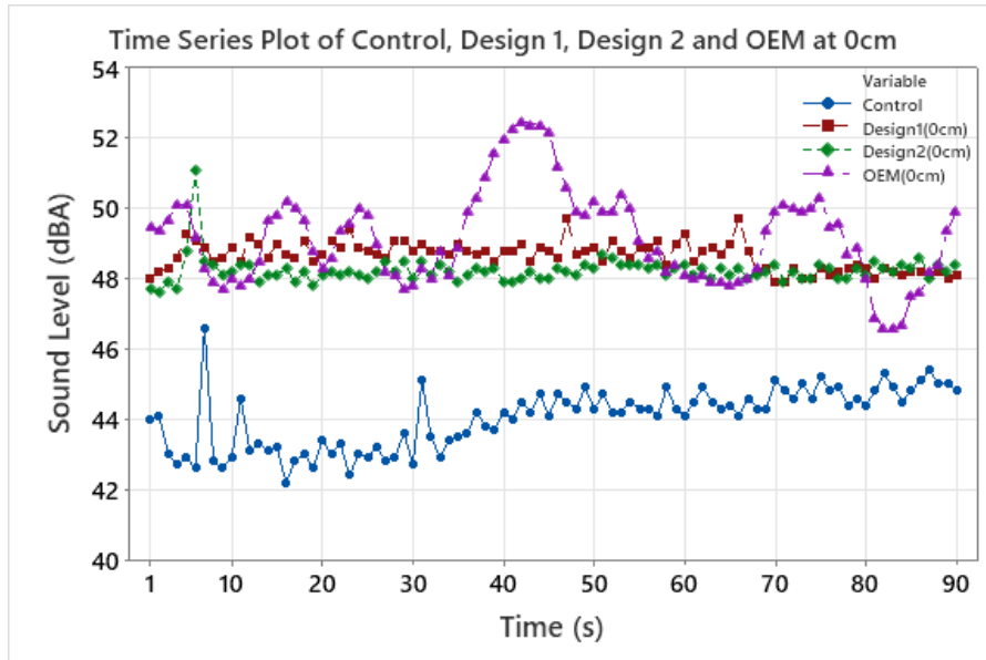
Fig. 9. Time plot of sound level measurements at 0 cm distance from outlet
