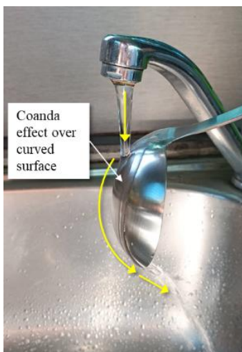
Fig. 1. Demonstration of the Coanda effect where water flow follows the curvature of the spoon.
